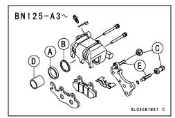
Install: Pad Spring [A] Caliper Holder [B] Pads and Caliper Pad Bolts
