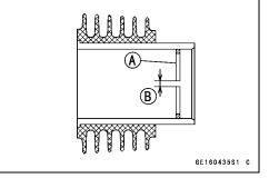
★ If the end gap of either ring is greater than the service limit, replace all the rings.
