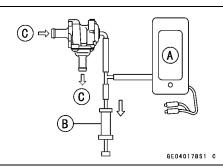
• Gradually raise the vacuum (lower the pressure) applied to the vacuum switch valve, and check the valve operation. When the vacuum is low, the vacuum switch valve should permit air to flow. When the vacuum raises to valve closing pressure, it should stop air flow.
