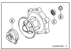
• Remove the hub bearings [A].
