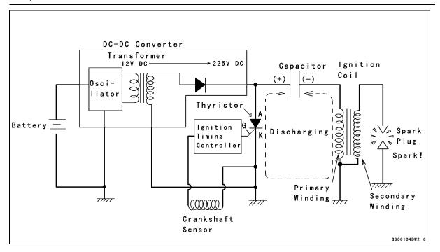
This sudden change in the primary current induces a primary voltage (counterelectromotive force) which is equal to the capacitor voltage (about 225 V) but against the discharging current. The primary voltage induces a high secondary voltage in the secondary coil, generating spark plug gap. The secondary voltage multiplied by winding ratio (about 90 : 1) reaches about 20 000 V.
