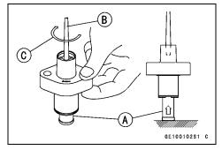
• While holding the rod in position with the screwdriver or a holder plate [A], install the tensioner on the cylinder block.
