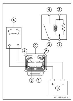
Starter Circuit Relay [A] Starter Relay [B] Interlock Diodes [C]
