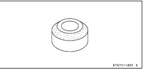
Valve Seat Cutter, 45° -  $\phi$ 32: 57001-1115
