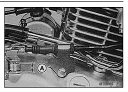
• Tighten the cover bolts and clutch cable holder bolts.
