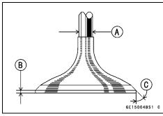
Valve Stem Diameter [A] Valve Head Thickness [B] 45° [C]
