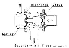
★ If the vacuum switch valve does not operate as described, replace it with a new one.
