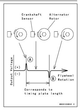
The crankshaft sensor, a signal generator, and voltage comparators determine the ignition timing in the ignition timing controller. The power supply circuit is the power source for the signal generator and the voltage comparators.
