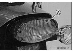
• Push the bulb [A] in the socket, turn it counterclockwise [B], and pull it out.
