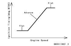
Before or after advancing period, the ignition timing is determined by the crankshaft sensor signal and the ignition timing remains constant.
