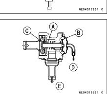
★ If the vacuum switch valve does not operate as described, replace it with a new one.
