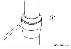
• Remove the retaining ring [A] from the outer tube with a screwdriver.
