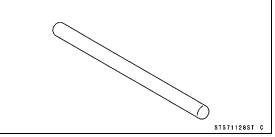
Valve Spring Compressor Adapter,  $\phi$ 22: 57001-1202
