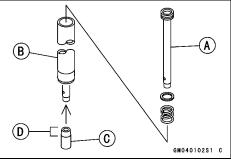
• Install the new guide bushing [A] with a used guide bushing [B] on it by tapping the used guide bushing with the fork oil seal driver [C] until it stops.
