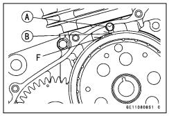
• Engage the camshaft sprocket [A] with the chain [B]. Then align the "T" mark [C] on the sprocket with the timing mark [D] on the cylinder head.
