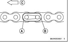
• Install the engine ground cable [A] as shown. Run the cable near the mounting boss [B].
