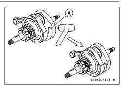
• Next, correct the vertical misalignment by either driving a wedge [A] in between the crank halves or by squeezing them in a vice, depending on the nature of the misalignment.
