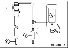
• Gradually raise the vacuum (lower the pressure) applied to the vacuum switch valve, and check the valve operation. When the vacuum is low, the vacuum switch valve should permit air to flow. When the vacuum raises to valve closing pressure, it should stop air flow.
