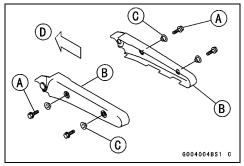
• Remove the seat bolts [A] and take off the seat [B].
